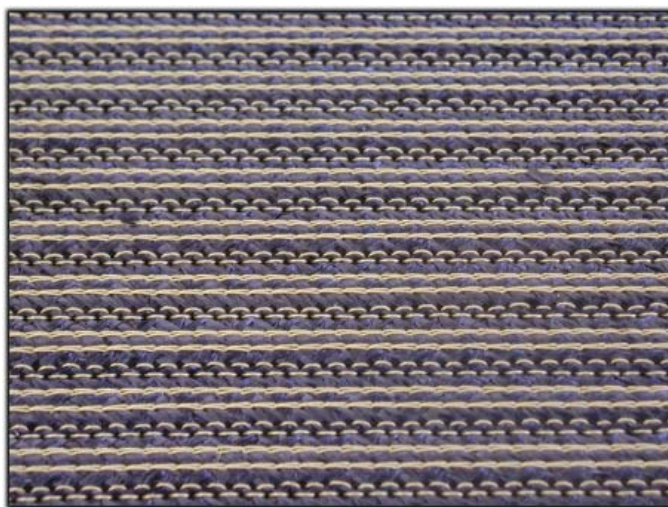
Figure 11 and 12- By chain stitch reinforced structure
